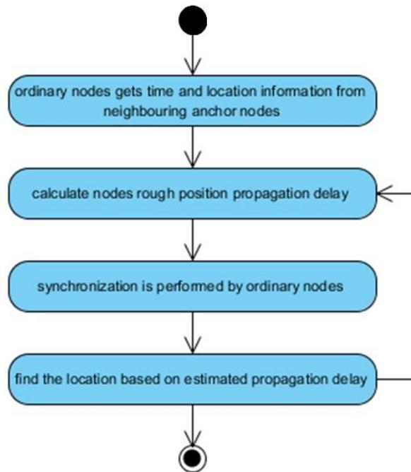
**Figure 2: Activity diagram of JSL algorithm.**
