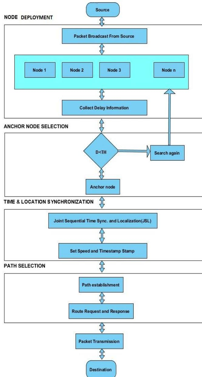
**Figure 1: Architecture for Reducing Propagation Delays in Underwater Sensor Networks.**
