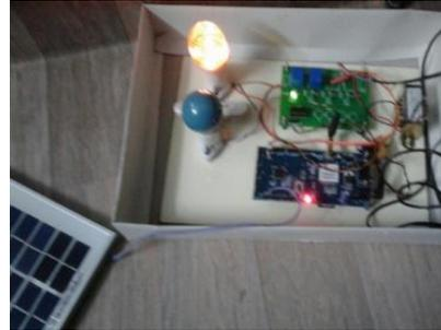
**Input01    Output Yellow(On)Green(Off)    Fig 2:Controlling of solar output through relays**
